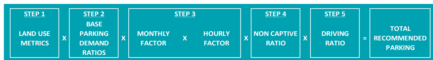
Figure 02: Shared Parking Steps
